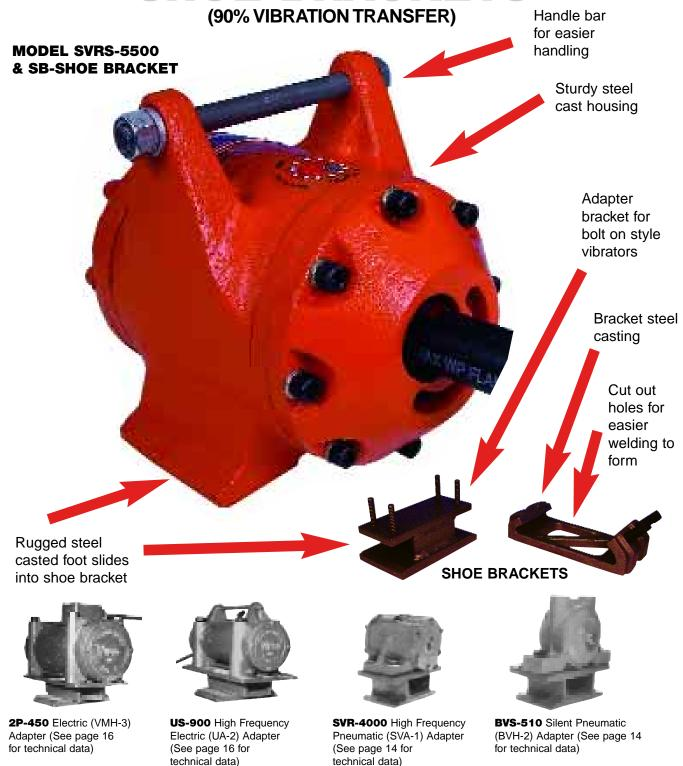
VIBCO's shoe brackets make portability easy with any type vibrator. A few are shown here, but practically any type vibrator can be used. Have VIBCO's engineers help you select a suitable vibrator for your application. SB shoe bracket is welded to channel stiffener or support beam. Vibrator with its adapter simply slides into bracket and is locked firmly by two hardened bolts.
