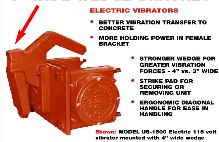
Use a mallet or hammer on VIBCO designed top strike pad to secure wedge into female bracket. (Usually only necessary when female bracket is worn.) To remove bracket use a mallet or hammer on bottom strike pad if wedge is pushed too far into female bracket.
